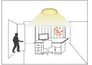
With movement and insufficient ambient lux level, the light is triggered on 100% by the detector.
